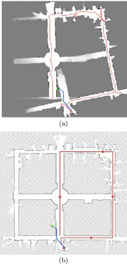
**Fig. 7** (a) Estimated map with: estimated robot position (red dot), estimated robot trajectory (red line), and planned robot trajectory (blue line); (b) Ground truth map with: actual robot position (red dot), real trajectory (red line), and planned trajectory (blue line).
