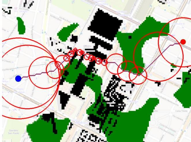
**Fig. 5.** Left: path creation. Buildings are shown in black; areas with low signal strength are shown in green; starting point is shown in blue, the goal is shown in red. Red circles show the minimum distance from obstacles for each waypoint.
